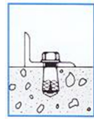
Anchor is set with bolt
