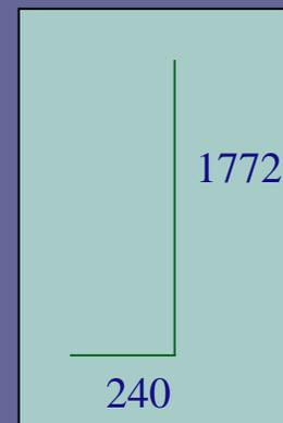
$$\begin{aligned} \text{根数: } N &= \text{排数} * [\text{Round}(\text{墙净长} - 50 * 2 / \text{间距}) + 1] \\ &= 2 * [\text{Round}(5200 - 50 * 2 / 200) + 1] \\ &= 2 * 27 \\ &= 54 \end{aligned}$$
