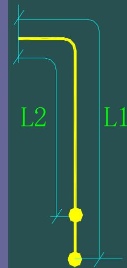
4b25:  $L2 = \text{层高} - (\text{本层楼面距接头距离} + \text{本层相邻纵筋交错距离}) - \text{梁高} + \text{柱头}$
